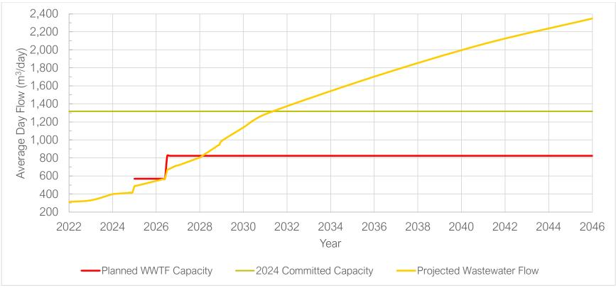
Figure 3-1 - Mount Brydges Wastewater Flow Projection
