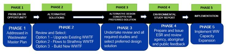
Figure 7-1: MCEA Flow Chart for Wastewater Treatment Capacity Solution in Mount Brydges
