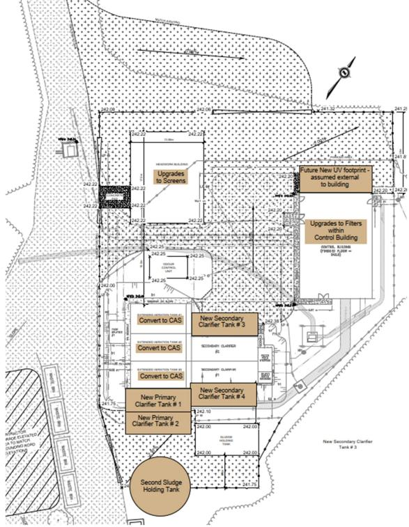
Figure 8-1 - Mount Brydges Treatment Capacity Option 1 Conceptual WWTF Site Layout
