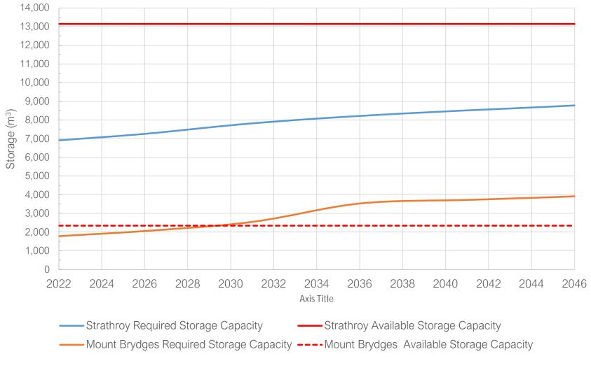
Figure 3-2: Strathroy and Mount Brydges Water Storage Projections
