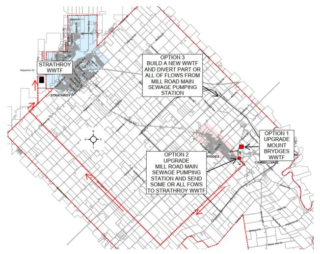
Figure 7-2: Mount Brydges Options to Increase Wastewater Capacity
