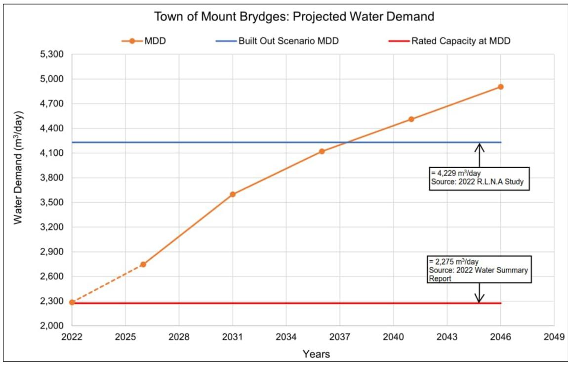
Rated Capacity to be confirmed in Water Master Plan
