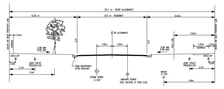
Figure 8-1- Current Strathroy-Caradoc Right of Way Standard
